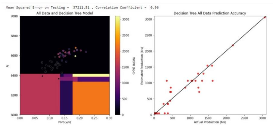
Nodes=3 MSE= 176144.81, Correlation Coefficient = 0.795 Nodes=5 MSE= 88694.48, Correlation Coefficient = 0.910 5 Nodes=10 MSE= 37211.51, Correlation Coefficient = 0.96
